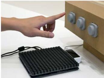
Figure 1b: The push button is rendered as a pulsing dot
