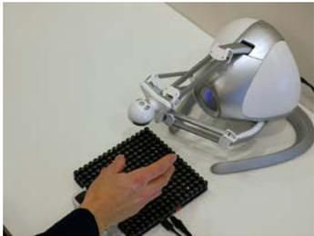
Figure 2a: As the robot end effector approaches the hand, the user perceives a tactile mid-air sensation
