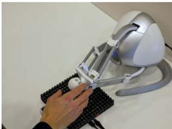
Figure 2b: This haptic feedforward allows the user to anticipate the robots action.
