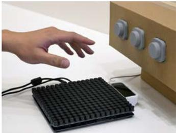
Figure 1a: As the user's hand moves towards a physical control, haptic aura conveys its functionality.
