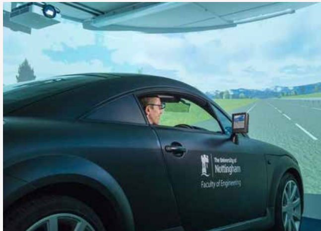
The study used a medium-fidelity driving simulator with a right-hand drive Audi TT car positioned within a curved screen.
